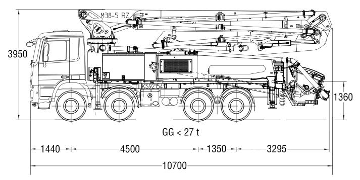
Note: Standard version. Dimensions and weights depend on truck, pump model and equipment. Dimensions in mm, MB-Actros 3241B(3244B)/8x4/45. For illustration only.
